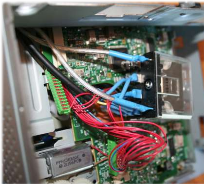
Image 4: Relay Being Installed
